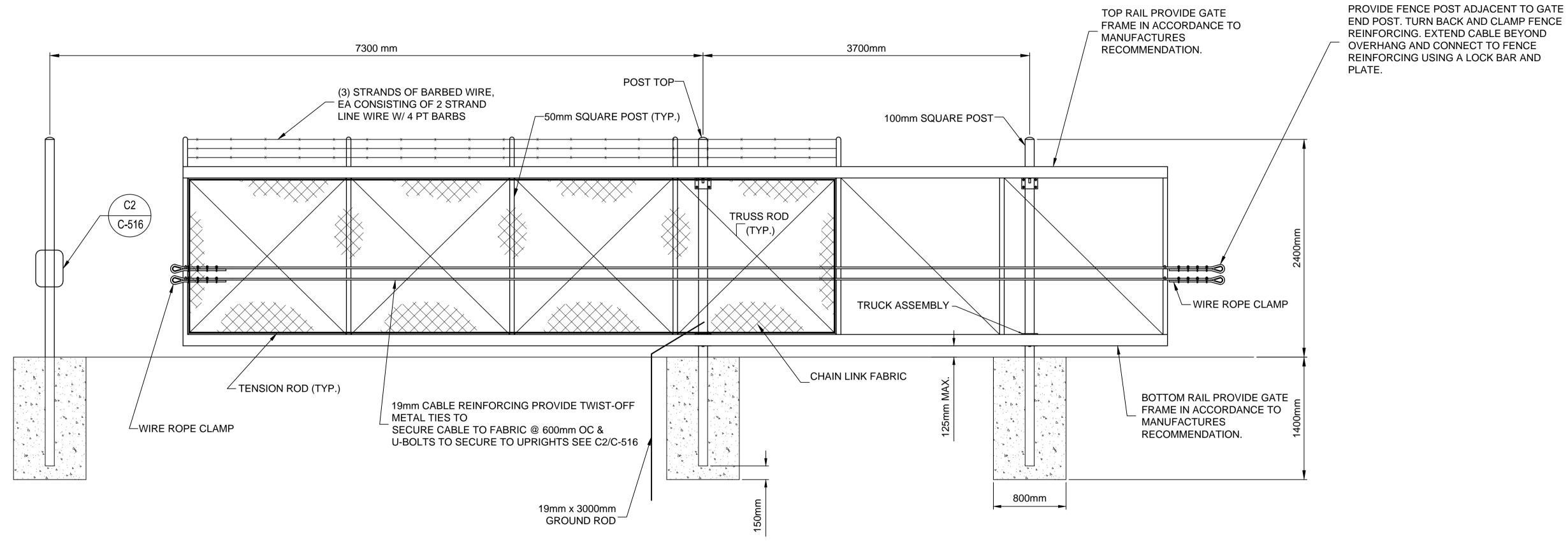
REINFORCING. EXTEND CABLE BEYOND OVERHANG AND CONNECT TO FENCE REINFORCING USING A LOCK BAR AND PLATE.
